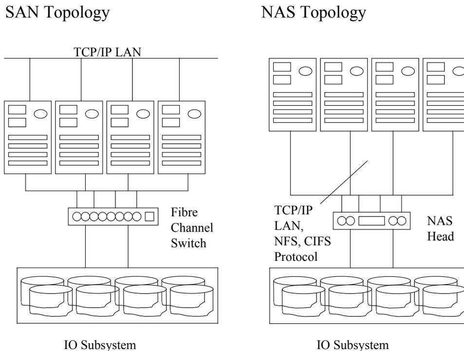
Most SAN versus NAS comparisons focus on the actual wires, but the argument can be made that the protocols are the most important factor that distinguish the two solutions. To illustrate, one thesis is that SCSI is faster than Ethernet, and hence reflects a better solution from a performance perspective. This statement is normally based on that fact that the TCP/IP overhead significantly impacts the efficiency of any data transfer scenario.
